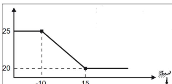
Figure 2: Temperature vs Static Pressure
