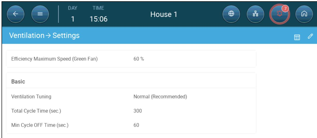
6. In Efficiency Maximum Speed, enter the fan's maximum speed (in percentage).
