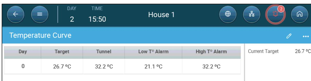
4. For each day, define the Tunnel temperature. This parameter defines the temperature at which Tunnel Mode begins to operate.
