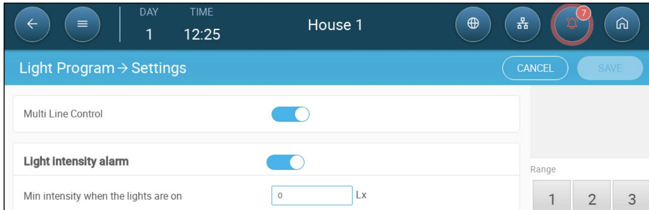
2. Define the minimum light intensity that lights must achieve. Below this level, Trio generates an alarm.
