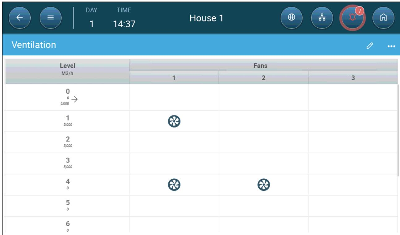
In this example Fan 1 operates according to the levels determined by the temperature and day, beginning at Level 1. The fan will supply up to 10% of the possible ventilation. At Level 4, Fan 2 also begins to operate, supplying up to 40% of the possible ventilation.
