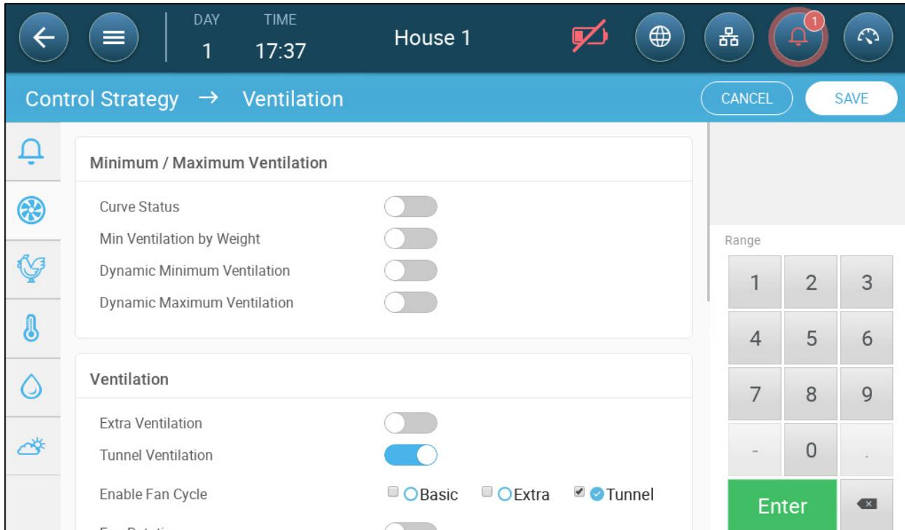
8. Under Enable Fan Cycle, check Tunnel.
