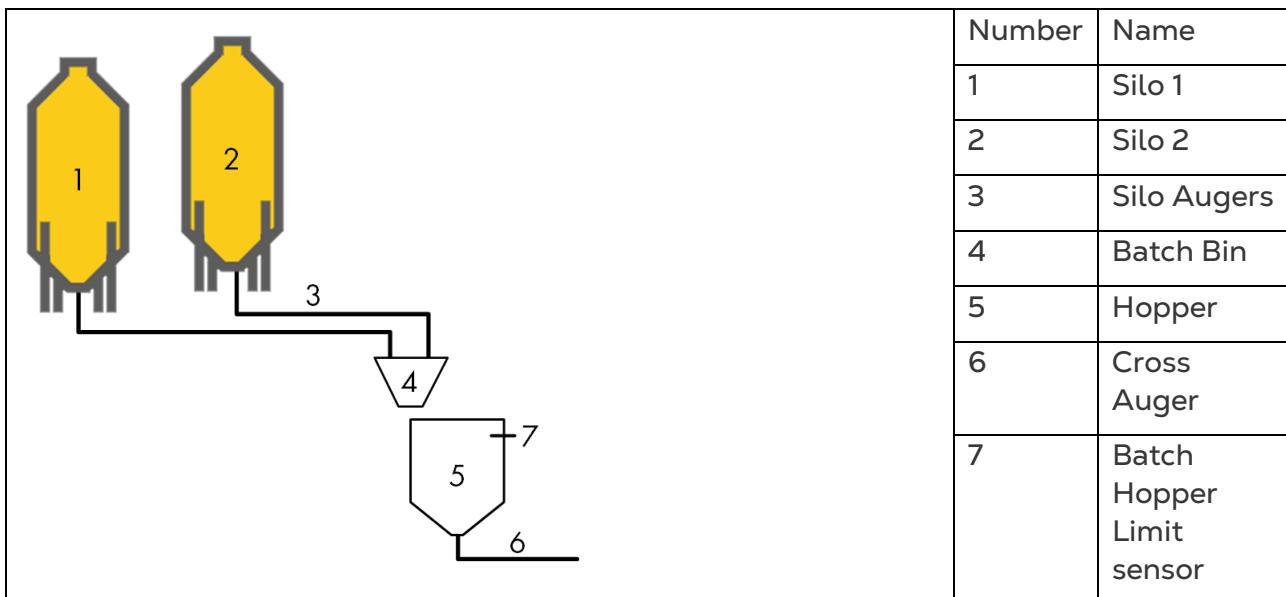
Figure 9: Batch Weighing System
