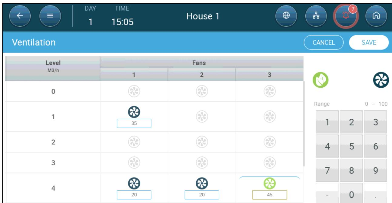
4. In the text box, enter the fan's minimum speed (in percentage).
