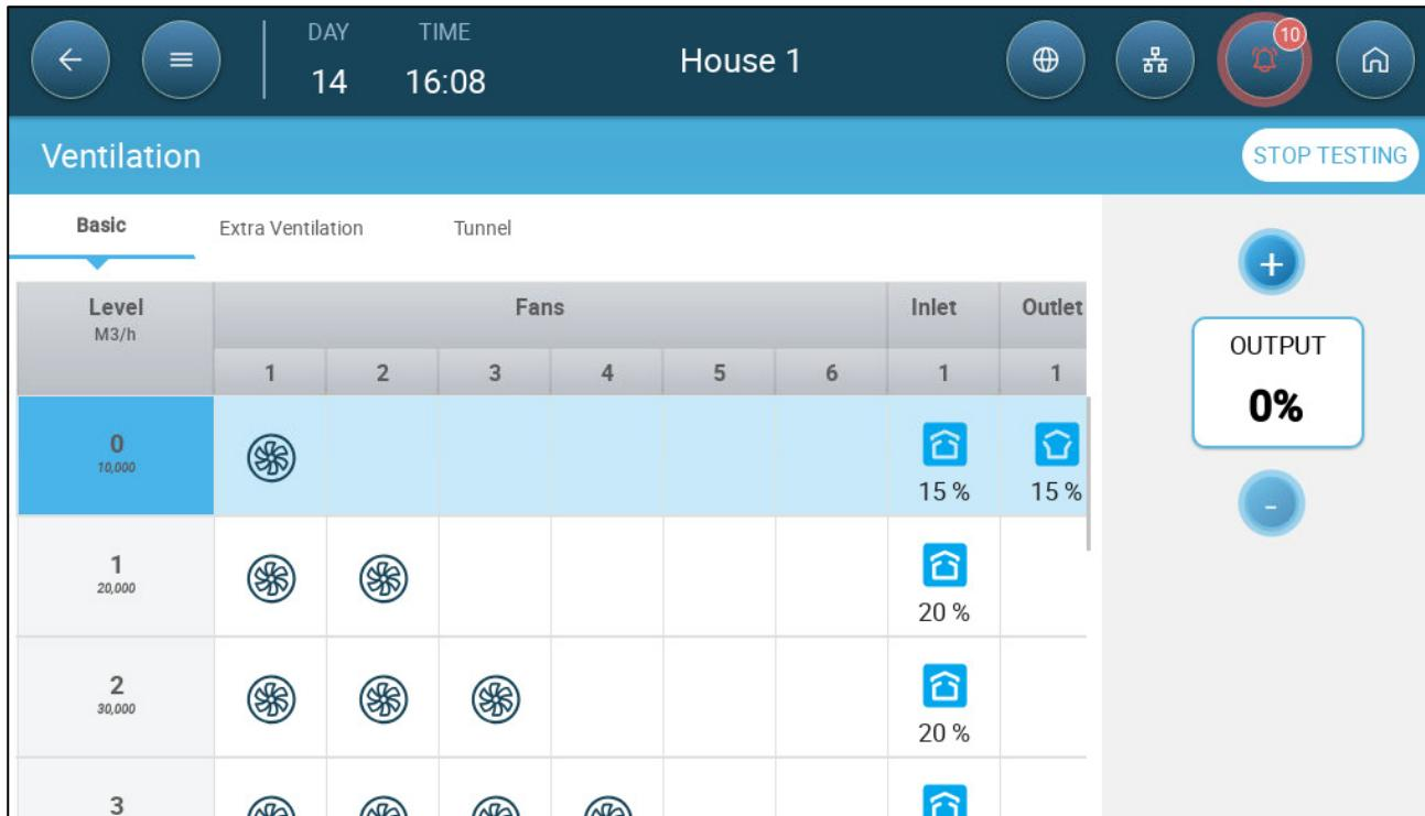
4. Testing begins at Level 0. Begin increasing the output. When the output increases to 10%, the ventilation level should rise to Level 1. When the output increases to 20%, the ventilation level should rise to Level 2.
