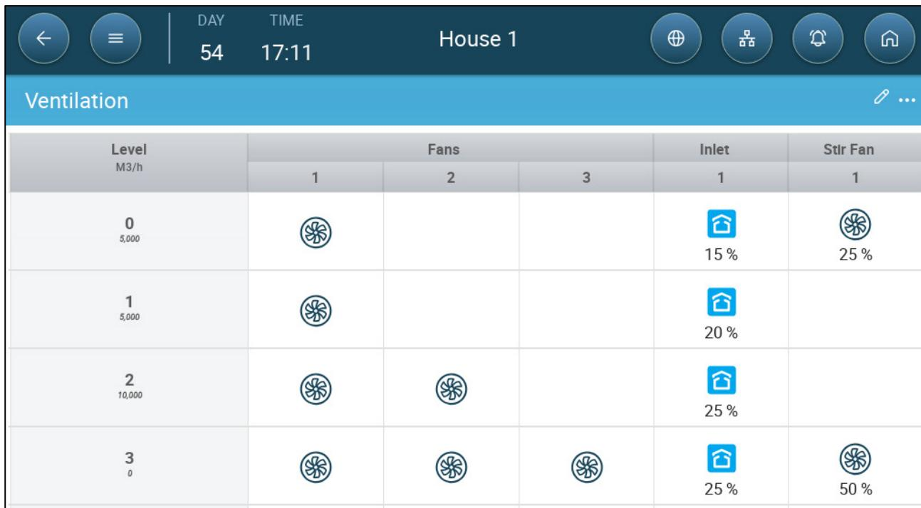
Figure 7: Variable Stir Fan Speed
