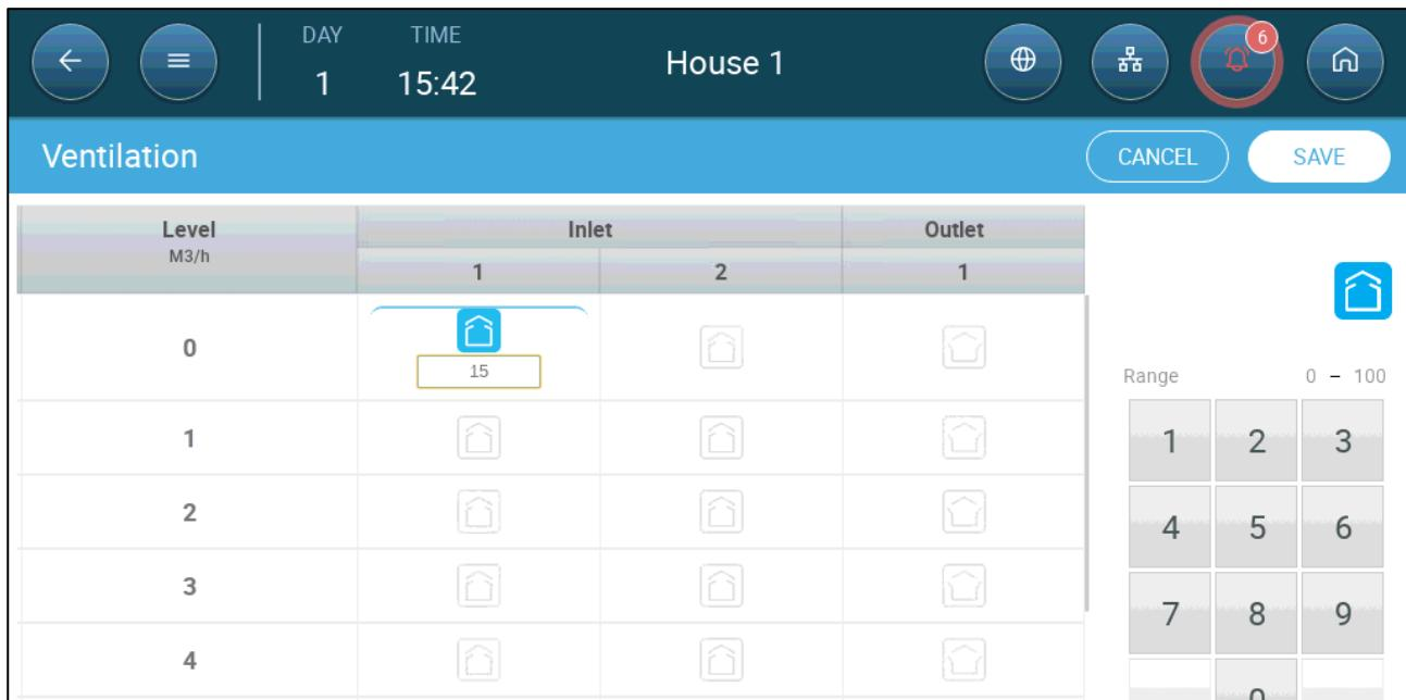
3. Click on a required inlet/outlet and enable it by clicking on the fan symbol that appears.
