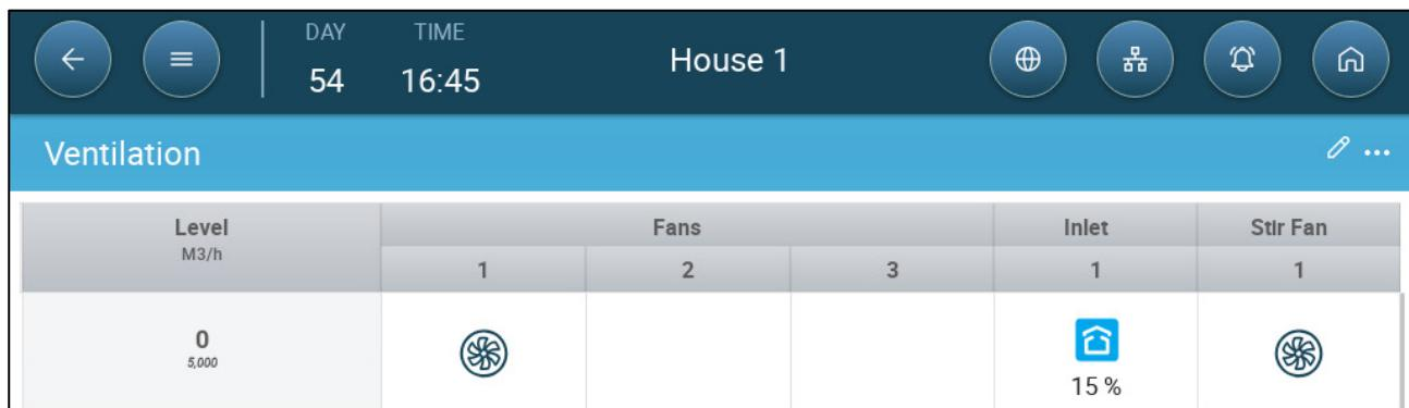
Figure 3: Valid Stir Fan – Exhaust Fan Configuration
