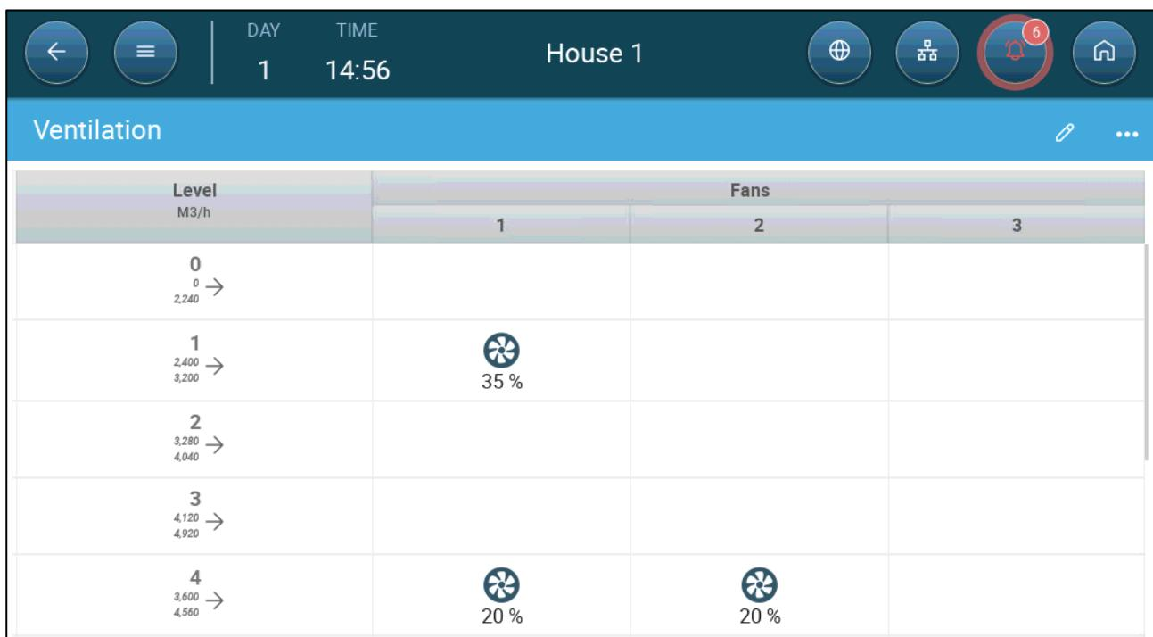
At Level 1 (10% output of the total fan capacity), Fan 1 runs at 35% speed. At Level 4 (40% of the total output), the speed drops to 20% but Fan 2 turns on as well.
