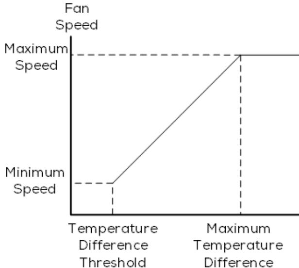
Figure 8: Variable Speed Stir Fan Speed vs Temperature
