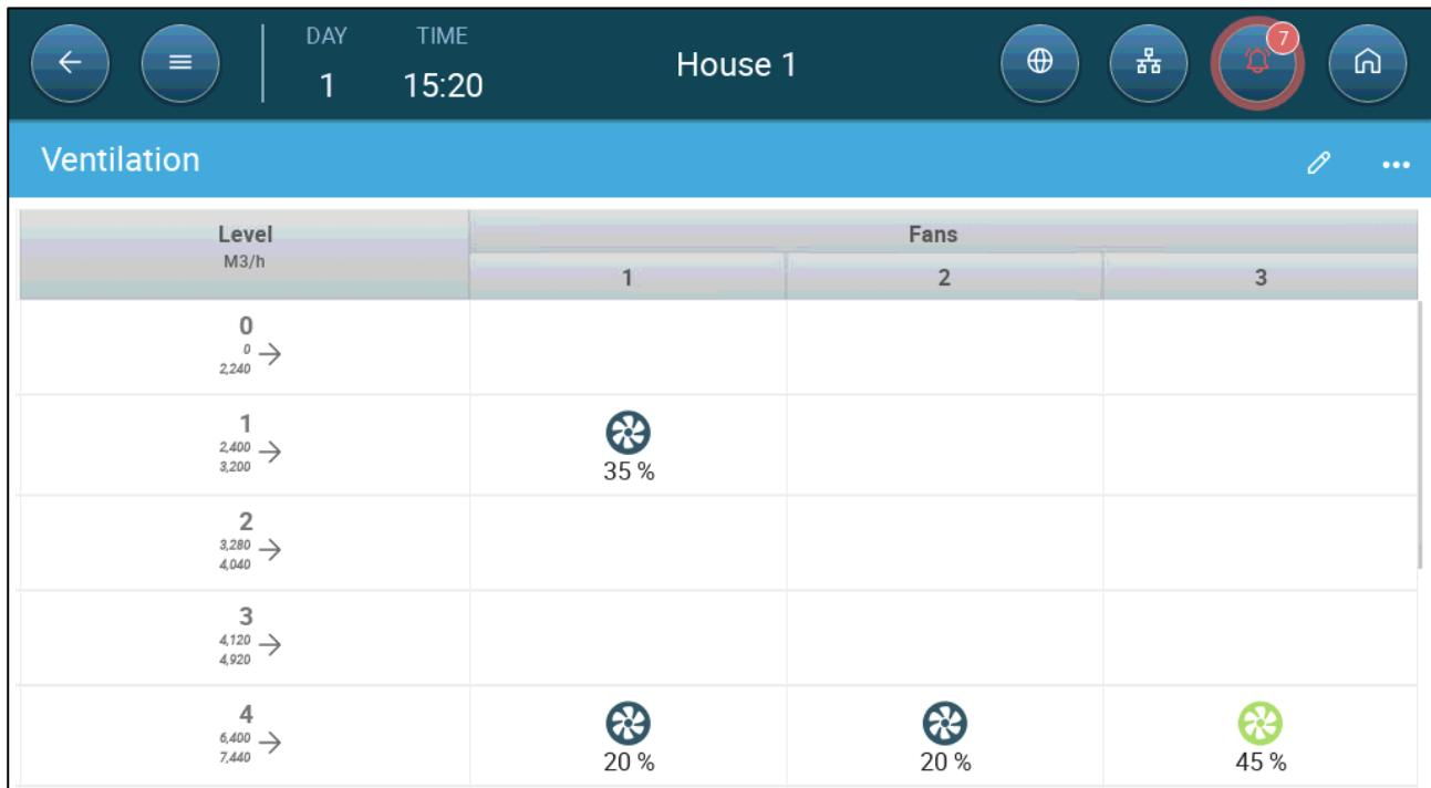
7. In this example Fan 1 and Fan 2 are standard analog fans, and Fan 3 is an efficiency fan whose minimum speed is 45% and maximum speed is 60% of the fan's possible speed. The ventilation capacity reflects the efficiency fan's capacity.
