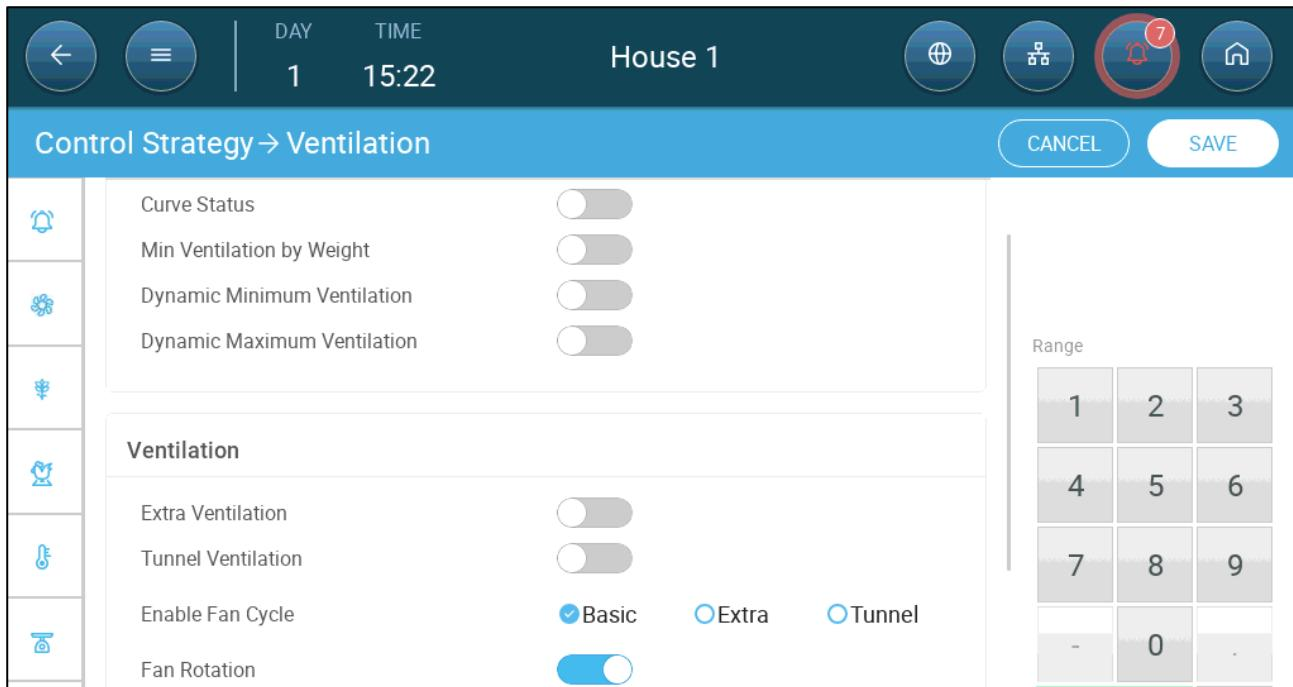
2. Enable Fan Cycle and Fan Rotation (Fan Rotation does not appear unless Fan Cycle is enabled.)
