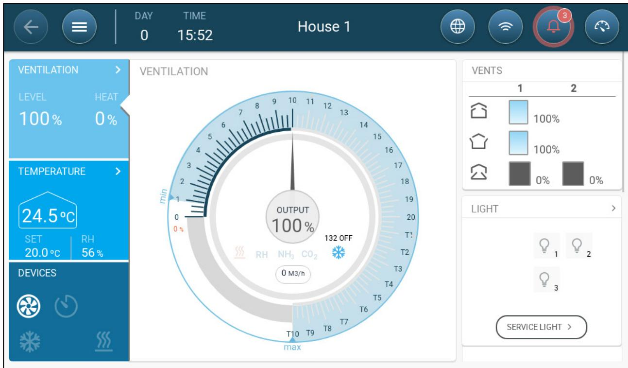
Service lights is a function that turns on the lights for a defined amount of time, temporarily overriding the programming. When the service light icon (which appears on the dashboard) is pressed, all lights are turned on.
