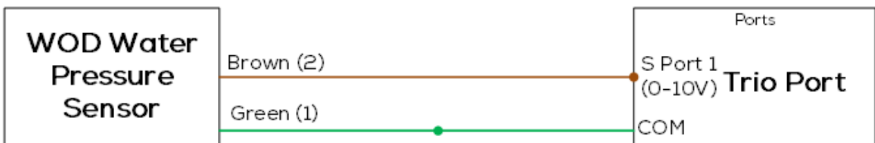
Figure 62: WOD Sensor Wiring Schematic
