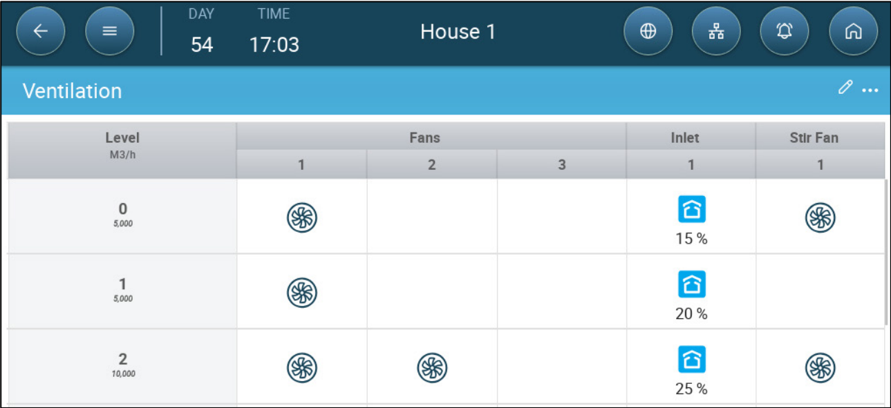
Figure 5: Change in Exhaust Fan – Stir Fan Continues Working
