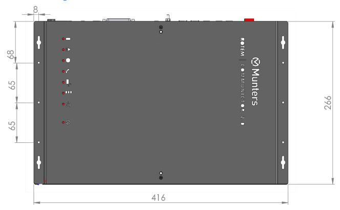
Figure 4: Dimensions (mm)
