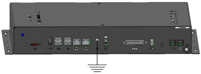
Figure 6: Grounding Schematic
