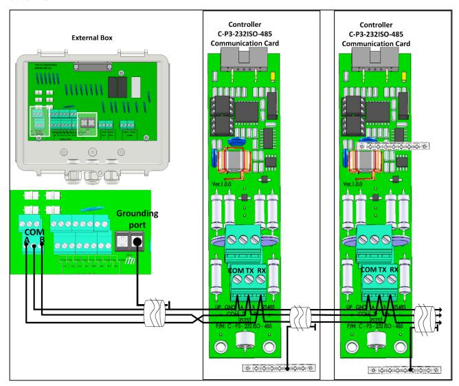
Figure 13: External Box – Controller Isolated RS-232 Connection
