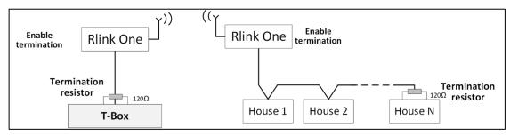
Figure 23: RLink One and House Termination
