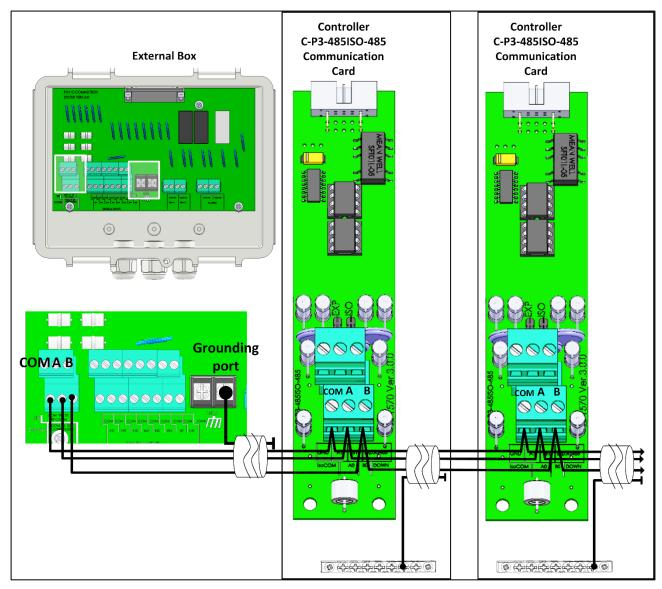
Figure 14: External Box – Controller RS-485 Connection
