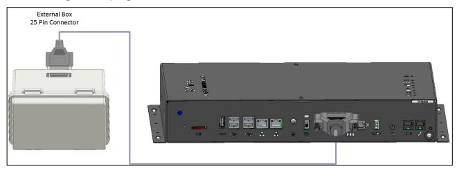
Figure 12: External Box – Communicator 2.0 Cable
