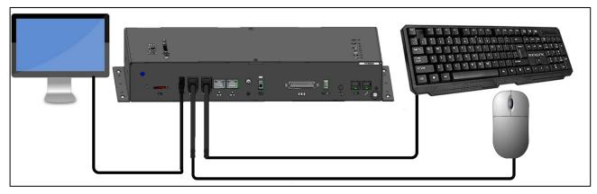
Figure 10: Connection to Peripherals
