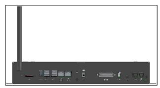
Figure 9: Antenna Attachment
