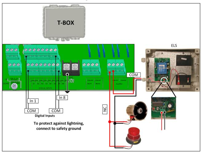
Figure 27: T-Box Wiring Diagram to ELS
