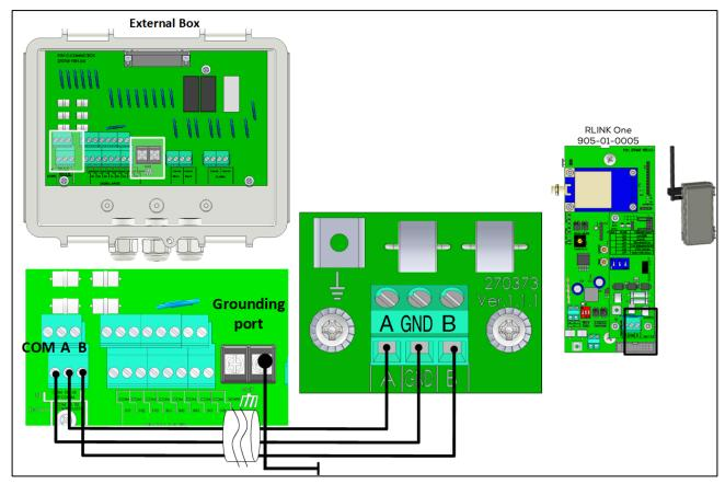
Figure 15: External Box – RLINK One Isolated RS-485 Connection
