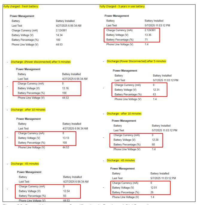
Figure 30: Power Management Specification in Fresh and Old Batteries
