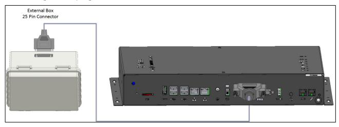
Figure 26: T-Box – Communicator 2.0 Connection
