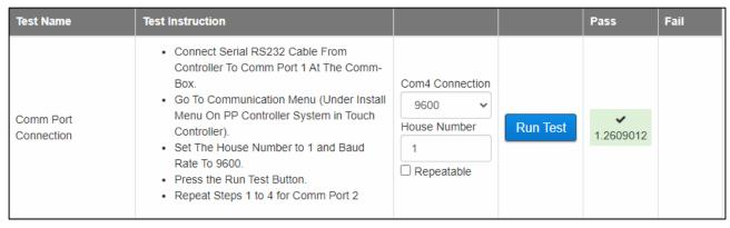
Figure 96: Standard Port Test
