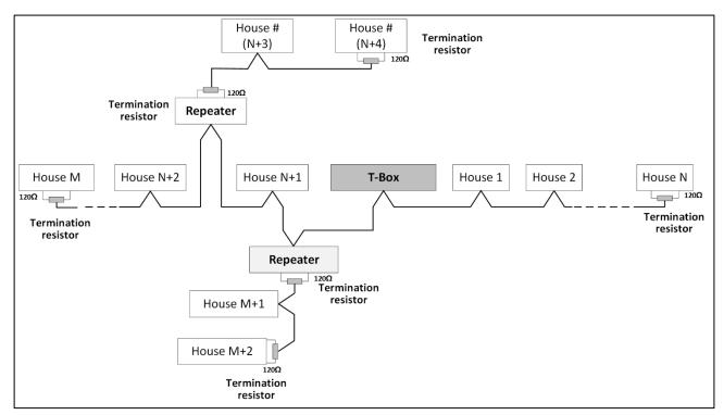
Figure 22: House and Multiple Repeaters Termination
