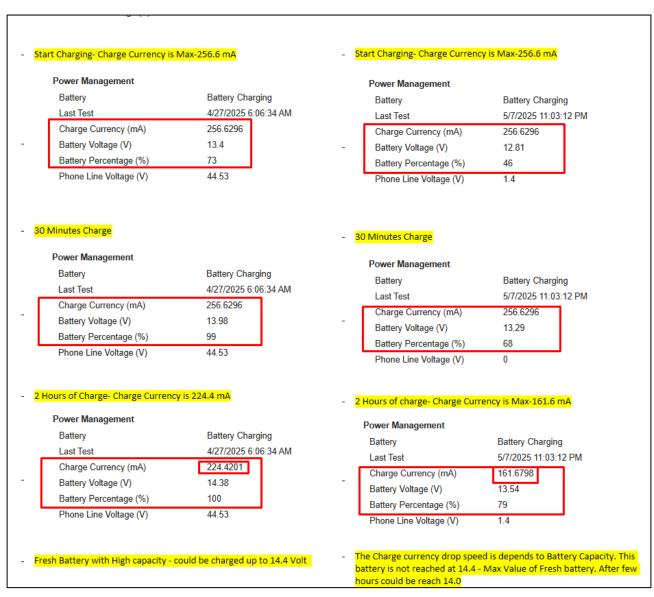
Figure 31: Power Management Specification in Fresh and Old Batteries (2)
