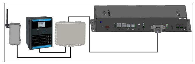
Figure 11: Communicator 2.0 – External Box – Controller/RLink One Block Diagram
