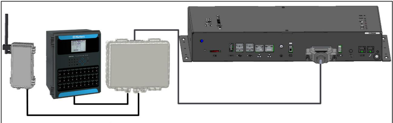
Figura 11: Communicator 2.0 Plus – External Box – Controller Block Diagram
