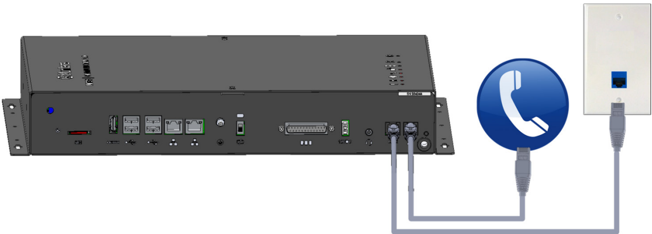
Figure 8: Phone Line Connection
