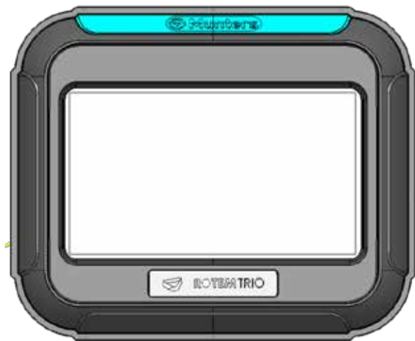
Figure 62: Trio CPU Panel, Front View
