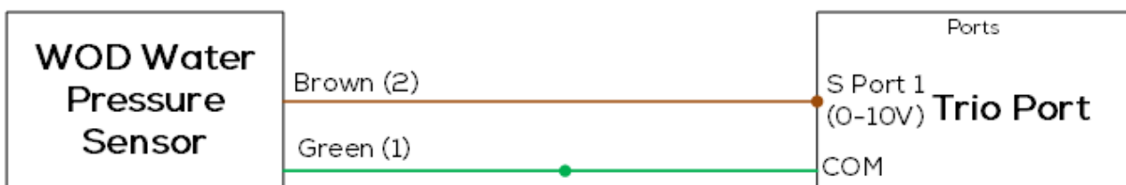
Figure 43: WOD Sensor Wiring Schematic
