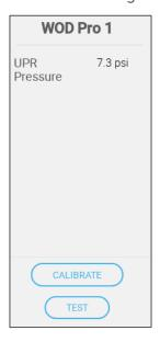
UPR Pressure: The UPR is a pressure regulator which has an adjustable range between 0 – 58 PSI.
