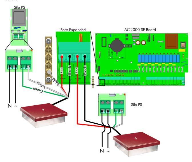
Connect Black and Red wires of Scale-1 > Scale 1 terminal, and Black and Red wires of Scale-2 > Scale 2 terminal
