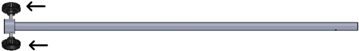
9. Place the two assembled tubes into the base rod; adjust to the required height and tighten the stoppers.
