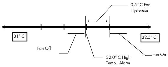
For this example the high temperature alarm is at 32.0°C. The fan is OFF when temperature is under 32.0°C and it is turned ON if the temperature goes above 32.5°C (High Temp + Hysteresis).
