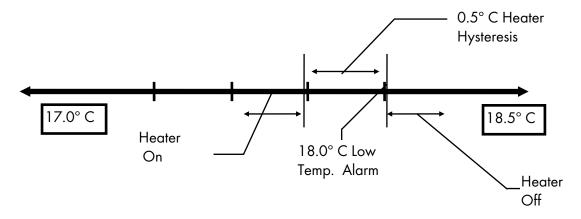
For this example the low temperature alarm is at 18.0°C. The heater is OFF when the temperature is superior to 18.0°C and it is turned ON if the temperature decreases less than 17.5°C (Low Temp - Hysteresis).
